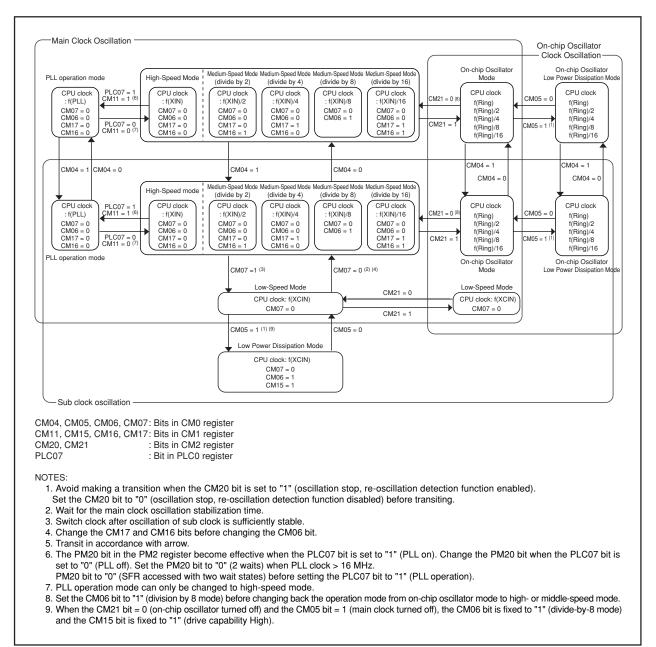
Figure 7.13 State Transition in Normal Operation Mode
